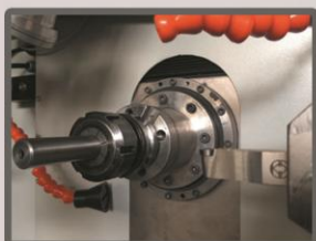
Rapid tool compensation by integral measuring system and wheel dressing unit.
